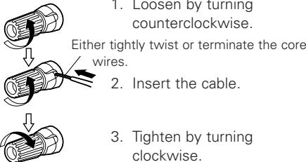
1. Loosen by turning counterclockwise.
